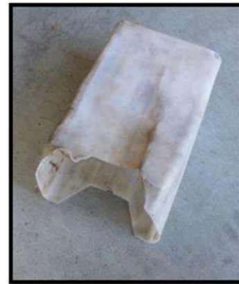
Figure 6 – Fire shelter high-density polyethylene plastic liner.
