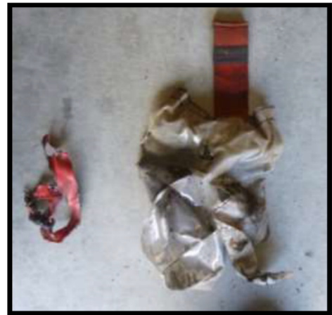
Figure 5 – Fire shelter pull-strip and PVC bag.
